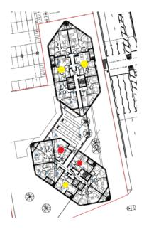
Fig 8 - Plan indicated the single aspect units which are either not north facing (yellow dot) or which are north facing (red dot) on typical floorplan.
